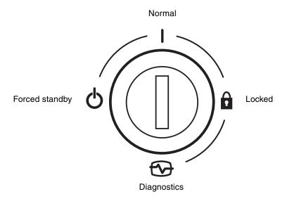
FIGURE 1-7 Keyswitch Positions (Sun Fire V240 Server)
