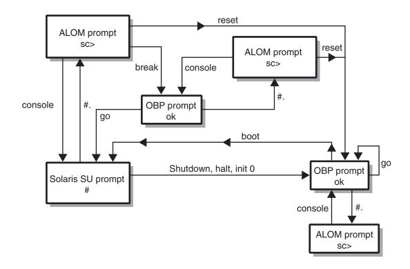
FIGURE 1-11 System Prompt Flow Diagram
