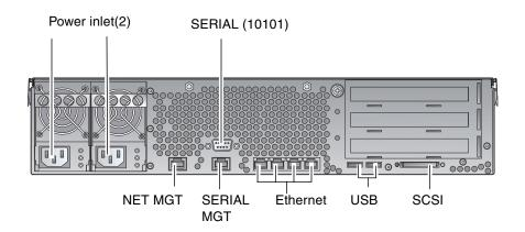
**FIGURE 1-9** I/O Ports (Sun Fire V240 Server)
