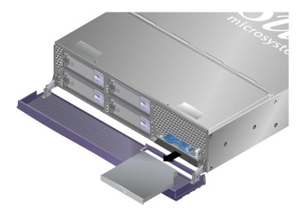
FIGURE 2-5 Removing a DVD-ROM Drive (Sun Fire V240 Server)
