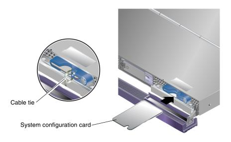
FIGURE 2-3 Inserting a System Configuration Card (Sun Fire V210 Server)
