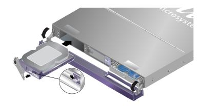
**FIGURE 2-4** Installing a Hard Drive (Sun Fire V210 Server)
