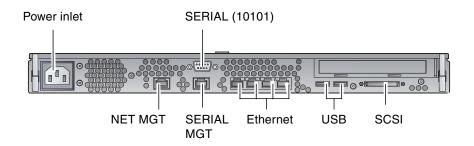
**FIGURE 1-8** I/O Ports (Sun Fire V210 Server)
