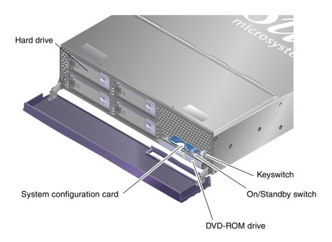
FIGURE 1-4 Location of Front Panel Features (Sun Fire V240 Server)
