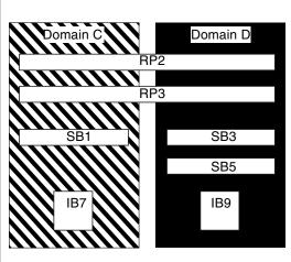
FIGURE 1-2 Sun Fire E6900 and 6800 Systems in Dual-Partition Mode
