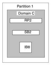
FIGURE 1-6 Sun Fire 3800 System in Dual-Partition Mode
