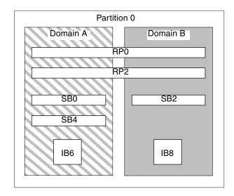
FIGURE 1-3 Sun Fire E4900/4810/4800 Systems in Single-Partition Mode
