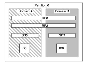
FIGURE 1-5 Sun Fire 3800 System in Single-Partition Mode
