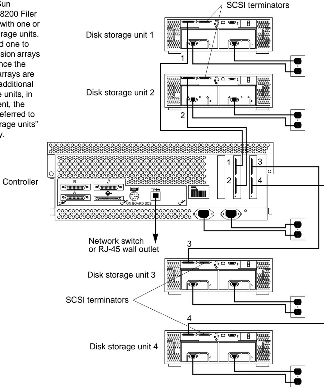
Controller SCSI connectors labeled in order of connection to disk storage units
