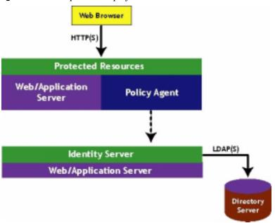
Figure 5-2 Simple Web Deployment Scenario
