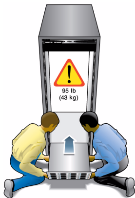
FIGURE 4 Installation du plateau
