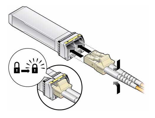
**Note** – The LC connector and SFP+ receptacles are keyed for proper fitting.
