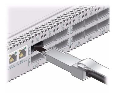
**Note** – On some QSFP cable connectors, there is a retraction strap. Both the retraction strap and L groove indicate the reference surface for the connector. When installing QSFP cables in the top row of receptacles (0A, 1A, 2A, and so on), ensure that the L groove and retraction strap are up. When installing QSFP cables in the bottom row of receptacles (0B, 1B, 2B, and so on) ensure that the L groove and retraction strap are down. See *Gateway Service*, identifying the data cable.
