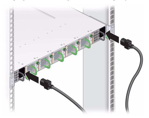
**4. Route the end of each power cord to its respective facility power receptacle.** Use cable ties or hook and loop fastener straps to bundle and secure the cord.
