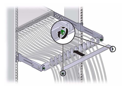
12. Route the data cables so that they do not interfere with other cables, or with servicing the gateway or other systems.
