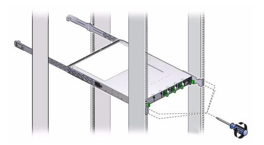
10. Install the cable management bracket to the tabs of the attachment brackets at the rear of the gateway, tightening the thumbscrews on each side of the cable management bracket.
