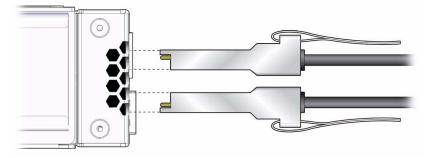
■ If the connector stops or binds after about 1/4 in. (5 mm) travel, back out and repeat from Step 6.
