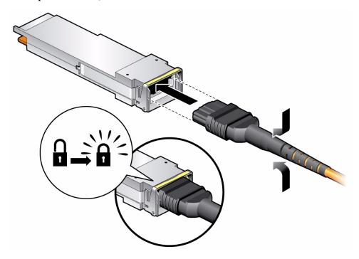
**Note** – The MTP connector and QSFP receptacle are keyed for proper fitting.
