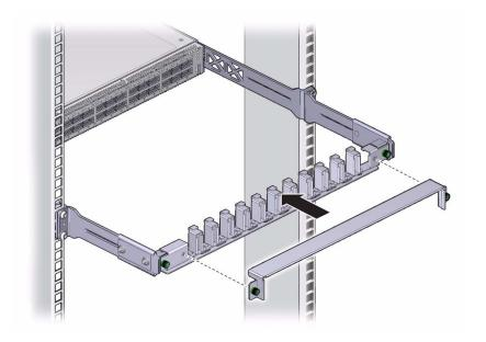
12. Tighten the thumbscrews on each side of the cover.
