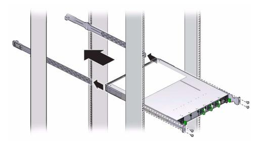
9. Mount the front of the gateway chassis to the front rack posts with two captive nuts and two screws at each side.
