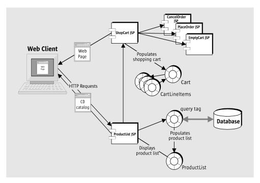
FIGURE 2-1 Architecture of the CDShopCart Application
