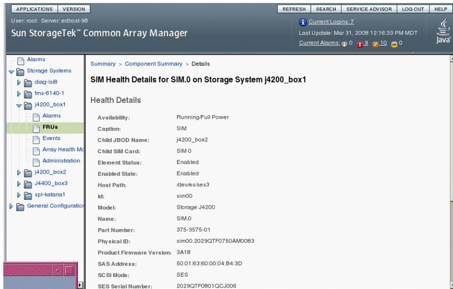
The screenshot displays the Sun StorageTek Common Array Manager interface. The main content area shows the 'SIM Health Details for SIM.0 on Storage System j4200\_box1'. The details are as follows:
