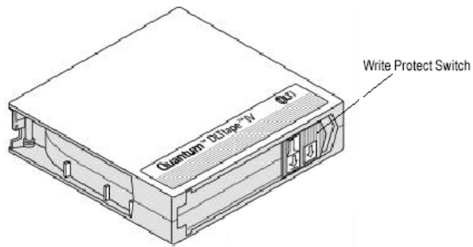
Figure B-5. Write-Protect Switch on Tape Cartridge
