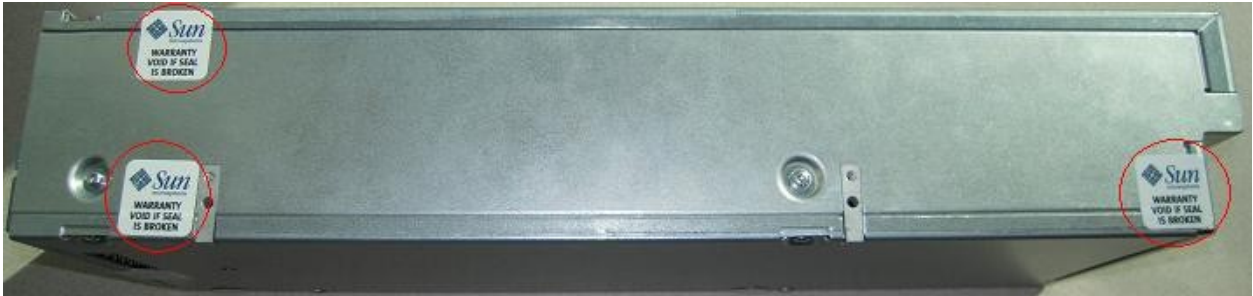
Figure 7: Tamper Evident Seals on Right Side
