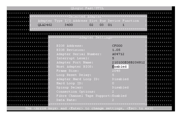
FIGURE 7-4 Example of the HBA BIOS Screen for an HBA WWN
