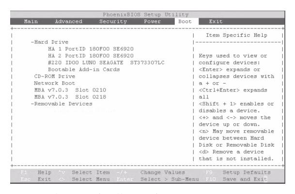
FIGURE 7-6 Example System BIOS for Enabling Booting from an FC LUN
