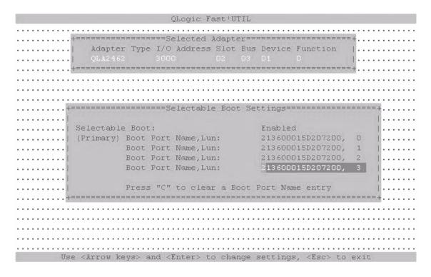
FIGURE 7-5 Example of the HBA BIOS screen for Enabling Boot from the FC LUN
