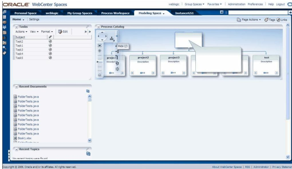
This page includes the Process Catalog, which graphically displays the various processes in the project. Each process is represented by a square. Navigation arrows within a given square enable you to find more information about the process it represents. The page also includes a number of panels that are standard to WebCenter.
