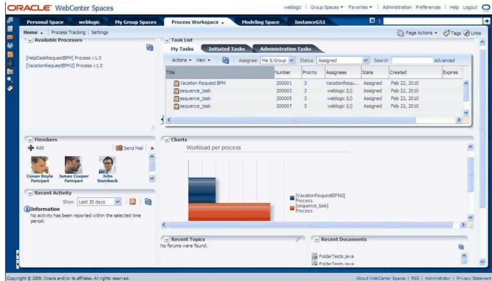
Included in the various panels of the Home page is the Available Processes panel, which displays the processes the user is authorized to execute. The Home page also displays the task inbox and dashboards (charts), and several standard panels of WebCenter.
