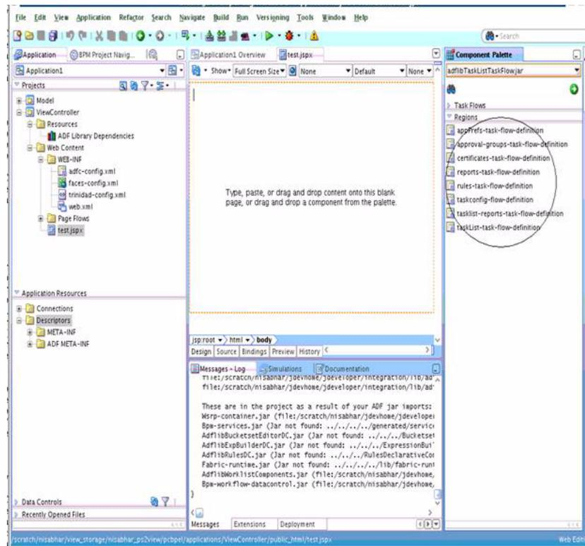
8. Drag and drop one of the Task Flow onto the JSPX page as a region. [Figure A-14](#) shows, by way of example, the TaskListTaskFlow being dropped onto the JSPX page as a region.
