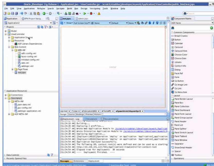
3. Drag and drop the Panel Splitter from the Component Palette into the JSPX page. The JSPX page now appears as shown in [Figure A-24](#).
