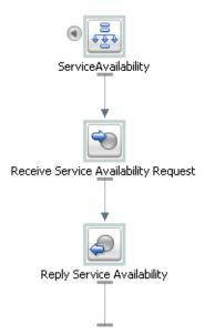
The Start Node contains both a Request Variable and a Response Variable that have been determined by the WSDL operation initially selected. The Receive receives the incoming request message (in this case for the three or fewer different kinds of cable service), and the Reply generates a response message and sends it back to the client.
