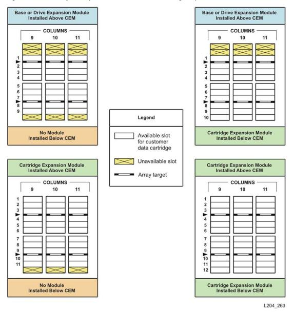
Figure 2–4 LTO-only Library Slots for Back Wall of Cartridge Expansion Module
