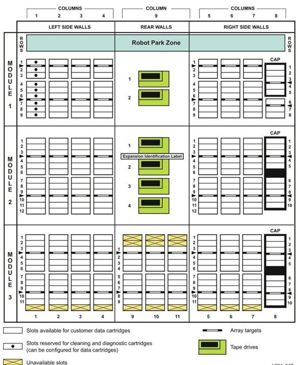
Figure 2–2 Firmware, LTO-only Library Slot Mapping
