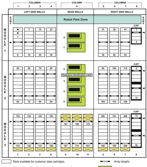
Figure 2–7 SCSI Mixed-Media Library Element Numbering Mapping
