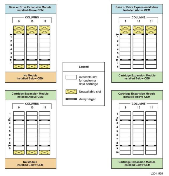
Figure 2–8 Mixed-Media Library Slots for Back Wall of Cartridge Expansion Module
