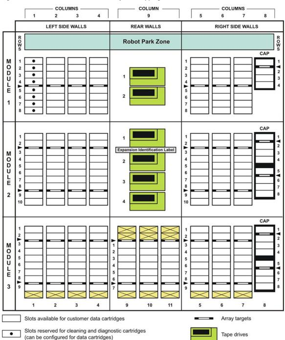
Figure 2–6 Firmware, Mixed-Media Library Slot Mapping
