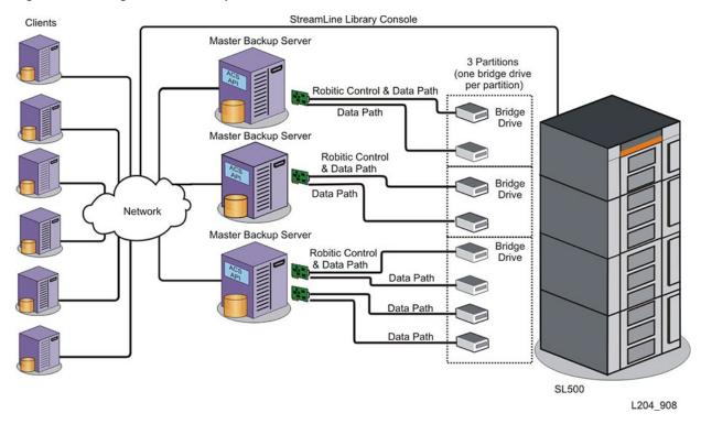
Figure 4–7 Bridged SL500 Example
