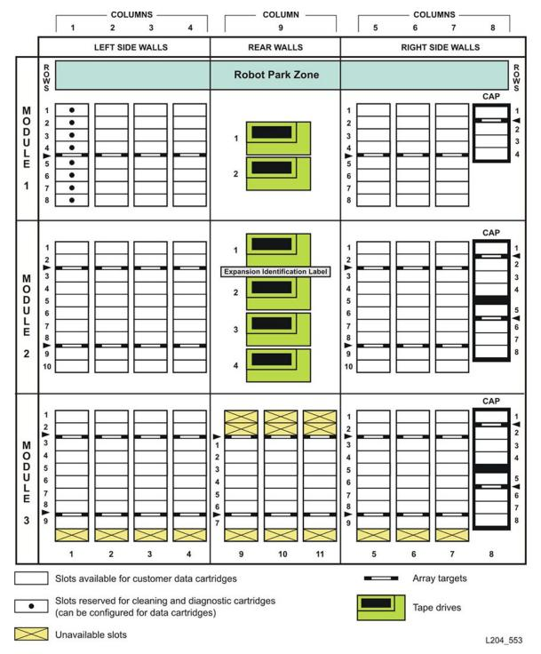
Figure 3–1 Slot Configuration for Partitioning Examples
