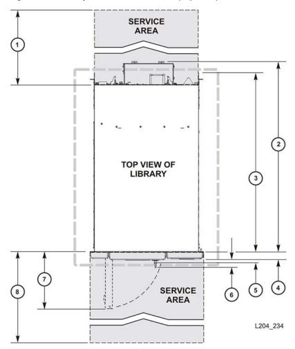
Figure 6–2 Library and Rack Dimensions (Top View)
