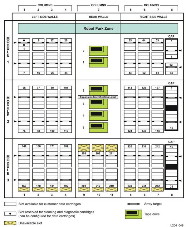
Figure 2–3 SCSI Element Numbering Mapping—LTO-only Library
