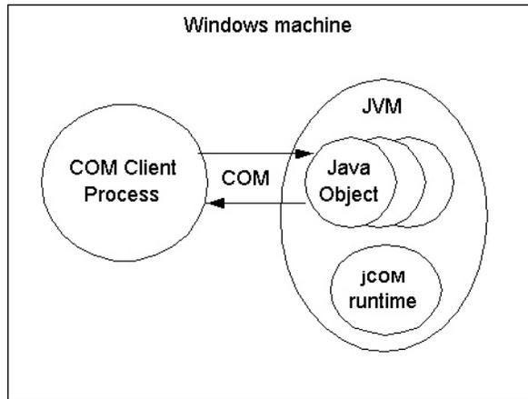
The JVM must call `com.bea.jcom.Jvm.register(<jvm id>)`, where `<jvm id>` is the id of the JVM as defined in `regjvm`.
