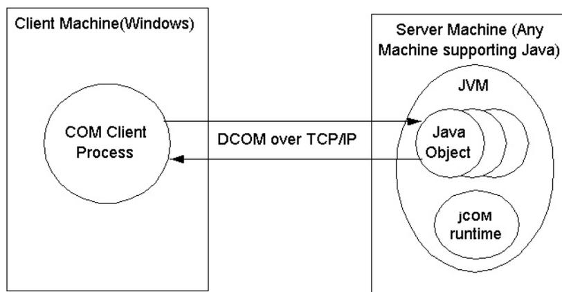
The Java code in the JVM must call `com.bea.jcom.Jvm.register(<jvm id>)`, where `<jvm id>` is the id of the JVM as defined in `regjvm`.
