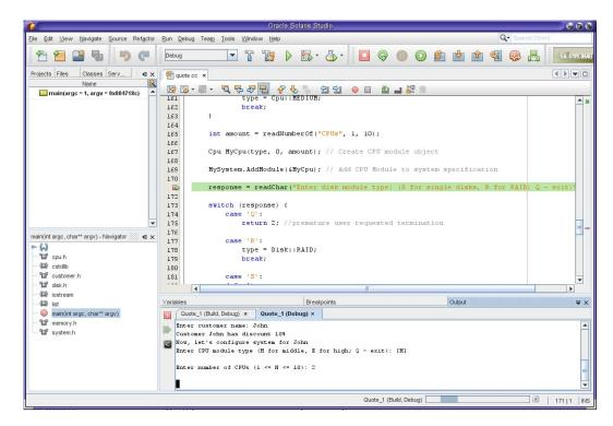
In the figure , the debugger is stopped at a breakpoint and the Output window shows the program interaction. Some debugger windows such as Variables and Breakpoints are also shown but not selected. You can open more debugging windows by selecting from the Window  $\rightarrow$  Debugging menu. One of the debugging windows is the Debugger Console window, which displays the interaction with dbx. You can also type commands at the (dbx) prompt in the Debugger Console window.
