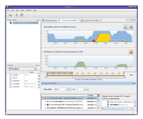
The figure shows the Process Tree Blocked Thread Details window at the bottom, which the user opened by clicking the lock icon in the Thread Microstates of Profiled Processes tool. On the right side of this window you can see the call stacks where the locks of the selected thread occurred.
