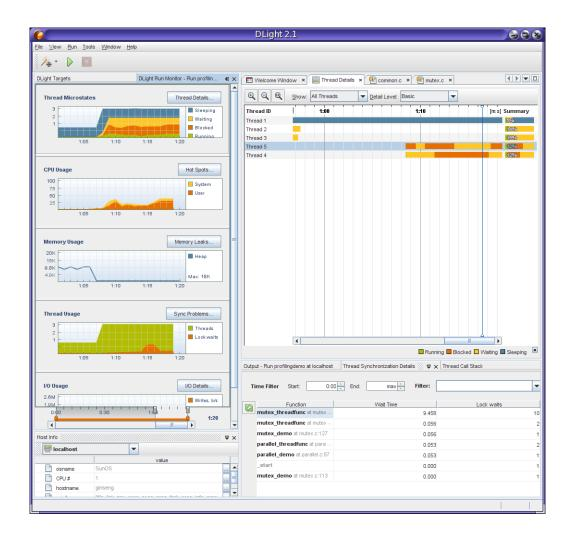
In the figure, the Thread Details window is open at the top left of the DLight window after the user clicked the Thread Details button in the Thread Microstates tool. The Thread Synchronization Details window, shown at the lower right, is open after the user clicked the Sync Problems button in the Thread Usage tool.
