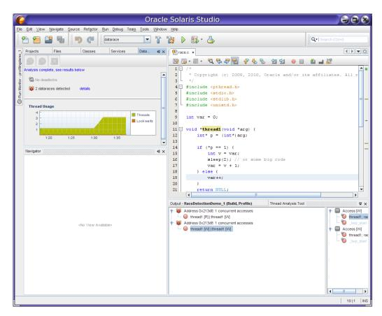
If you click the details link in the Data Race Detection window, the Thread Details window opens to show where the data races occur. You can double-click the threads in the Thread Details window to open the source file where the problem occurs and go to the affected line of code.
