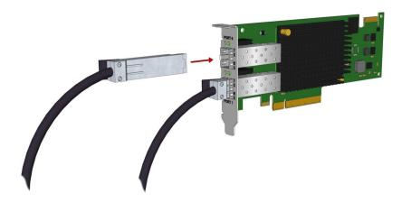
2. After the copper cables are connected to the HBA, insert the other end of the cables into the empty SFP+ cages on FC devices.
