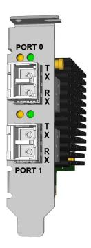
Each port has a corresponding set of LEDs that provide a visual indication of the operating state.
