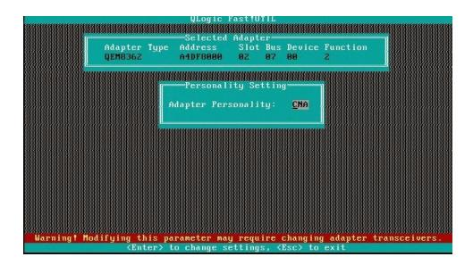
Press Enter to change the operating protocol mode (The Enter key toggles the operating protocol mode between FC and CNA.), or press the Esc key to keep the displayed mode.
