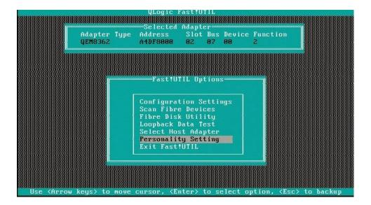
The current operating protocol mode of the universal HBA (either FC or CNA) is displayed, as shown in the following figure. If the current operating protocol mode is correct, skip to step 6. If the current operating protocol mode is incorrect, continue to step 5.
