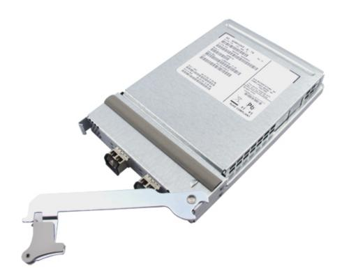
6. Insert the universal HBA into an empty PCI ExpressModule slot.
