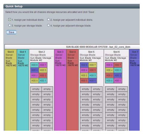
**Note** – Empty slots shown in the Quick Setup dialog represent chassis blade slots that are empty (nothing installed).
