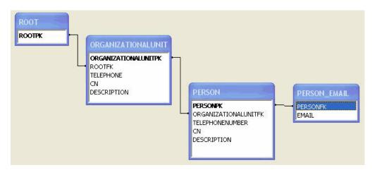
This graphic shows the relational structure created by the LDAP to relational mapping process from the LDAP tree example.
