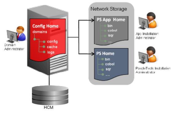
Example: Typical Decoupled Deployment
