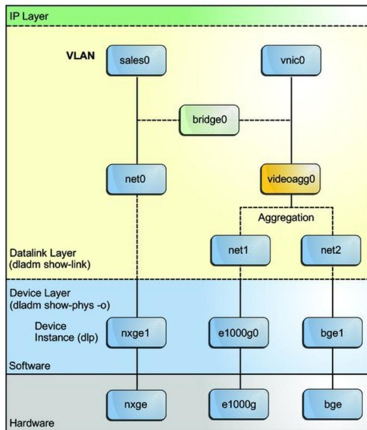
Two interfaces, **net0** and **videoagg0**, are configured as a bridge, **bridge0**. Packets that are received on one interface are forwarded to the other interface. After the bridge configuration, both interfaces can still be used to configure VLANs and IP interfaces.
