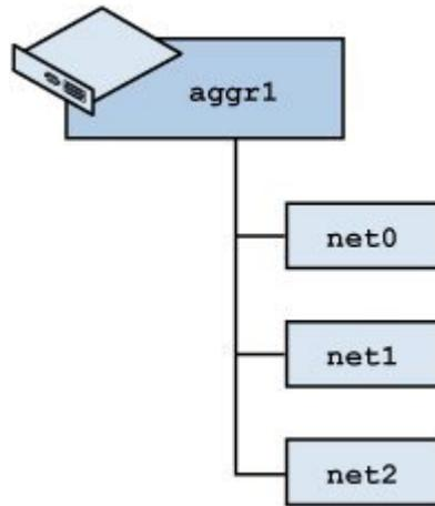
The illustration shows an aggregation `aggr1` that consists of three underlying datalinks, `net0`, `net1`, and `net2`. These datalinks are dedicated to serve the traffic that traverses the system through the aggregation. The underlying links are hidden from external applications. Instead, the logical datalink `aggr1` is accessible.
