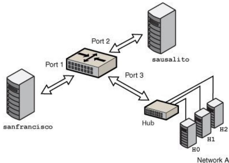
The bridge, `goldengate`, is an Oracle Solaris system that has bridging configured. The systems `sanfrancisco` and `sausalito` are physically connected to the bridge. Network A uses a hub that is physically connected to the bridge on one side and to three computer systems on the other side. The bridge ports are the links `net0`, `net1`, and `net2`.
