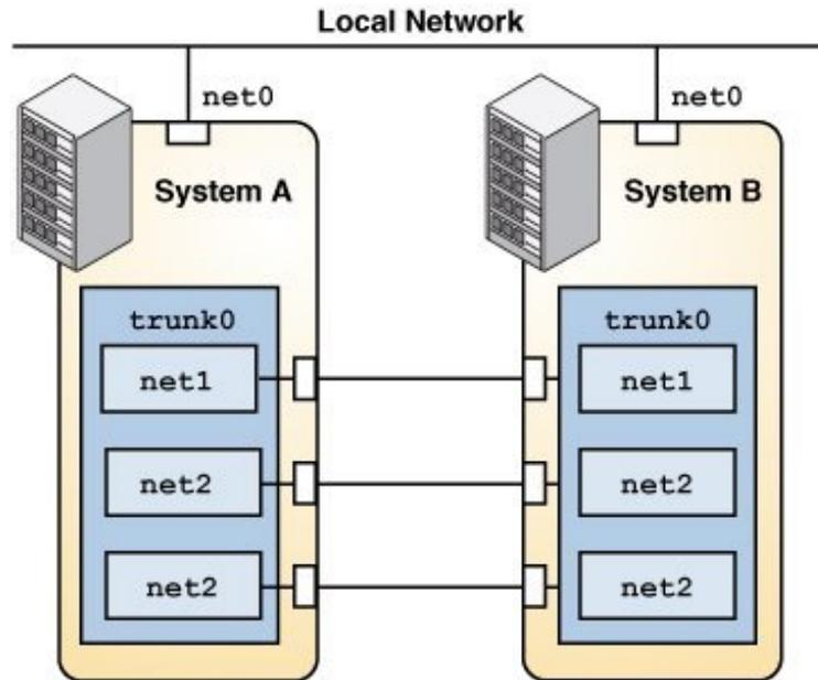
The illustration shows trunk aggregation `trunk0` on System A directly connected to trunk aggregation `trunk0` on System B by means of the corresponding links between their respective underlying datalinks. This setup enables Systems A and B to provide redundancy, high availability, and high-speed communication between both systems. Each system also has `net0` configured for traffic flow within the local network.
