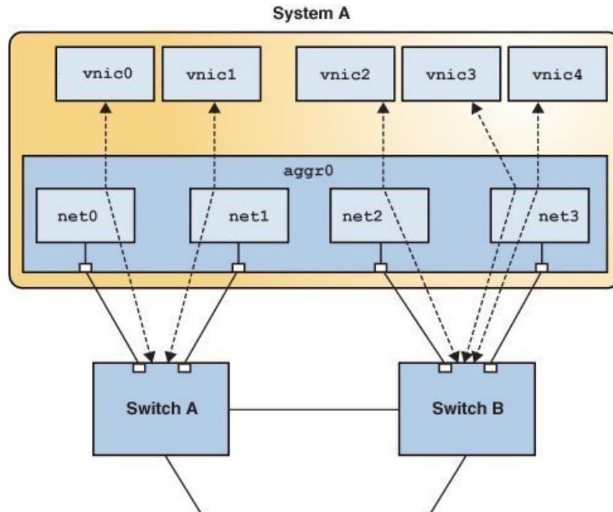
The figure shows System A with link aggregation `aggr0`. The aggregation consists of four underlying links, from `net0` to `net3`. VNICs `vnic0` through `vnic4` are also configured over the aggregation. The aggregation is connected to Switch A and Switch B, which in turn connect to other destination systems in the wider network.
