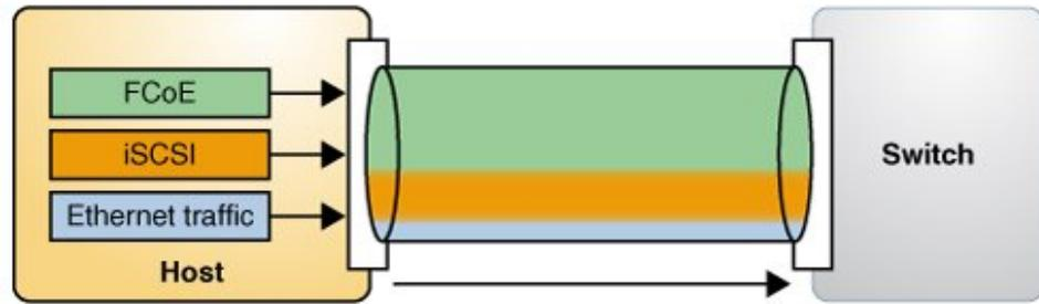
The host in the figure has different types of traffic, such as FCoE and iSCSI, that share the link bandwidth. In the figure, the priority and bandwidth as shown in the following table are assigned for different types of traffic.
