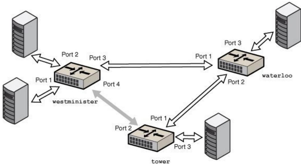
The figure shows a bridged network that is configured in a ring. The configuration shows three bridges. Two systems are physically connected to the westminister bridge. One system is physically connected to the waterloo bridge and one system is physically connected to the tower bridge. The bridges are physically connected to each other through the bridge ports.
