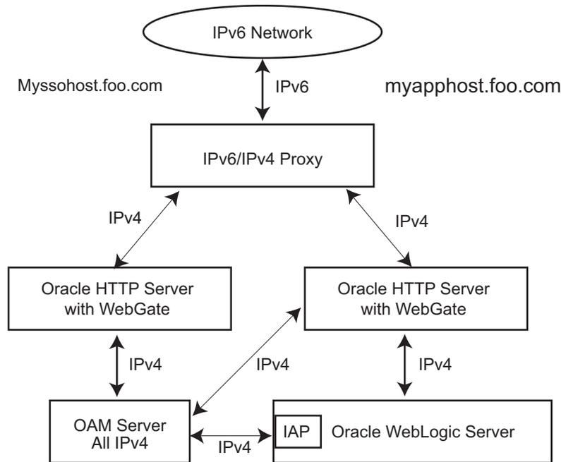
As illustrated in [Figure 15–3](#), the IPv6 network communicates with the IPv6/IPv4 proxy, which in turn communicates with the Oracle HTTP Server using IPv4. WebGate, Oracle Access Manager server, and Oracle WebLogic Server with the Identity Asserter all communicate with each other using IPv4.
