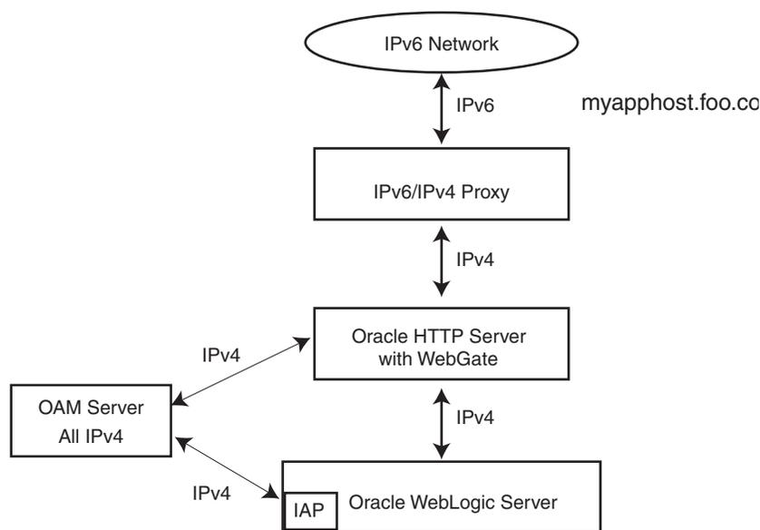
As illustrated in Figure 15–2, the IPv6 network communicates with the IPv6/IPv4 proxy, which in turn communicates with the Oracle HTTP Server and WebGate using IPv4. WebGate, Oracle Access Manager servers, and Oracle WebLogic Server with the Authentication provider all communicate with each other using IPv4.
