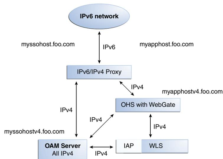
As illustrated in [Figure 15–2](#), the IPv6 network communicates with the IPv6/IPv4 proxy, which in turn communicates with the Oracle HTTP Server using IPv4. Webgate, OAM Server, and Oracle WebLogic Server with the Identity Asserter all communicate with each other using IPV4.
