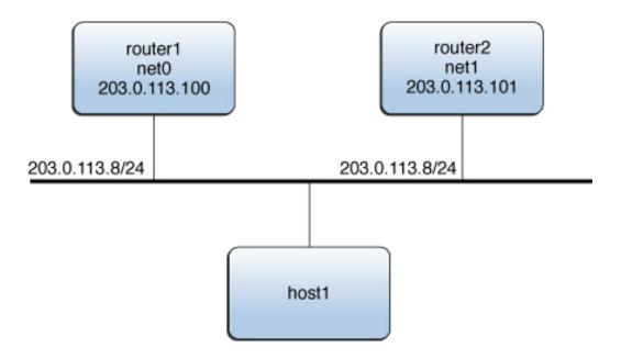
In this example, the IP address 203.0.113.8 is configured as the default gateway for host1. This IP address is the virtual IP address that is protected by the virtual router that is configured on two routers: router1 and router2. At any given time, only one of the two routers serves as the master router, which assumes the responsibilities of the virtual router and forwards packets that come from host1.
