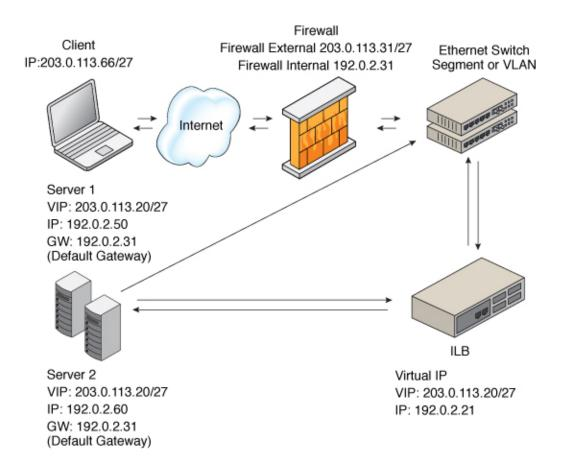
In this figure, both back-end servers are in the same subnet (192.0.2.0/27) as the ILB box. The servers are also connected to the router so that they can reply directly to clients after receiving a request forwarded by the ILB box.
