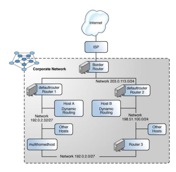
Router 2 contains two wired network connections, one connection to network 198.51.100.0 and one to network 203.0.113.0. The example shows how to configure a system as a router (Router 2) of the 198.51.100.0 network.
