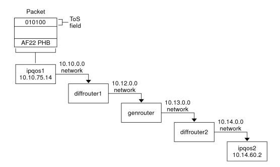
The flow of the packet that is shown in this figure begins with the progress of a packet that originates at host ipqos1. The steps then continue through several hops to host ipqos2.
