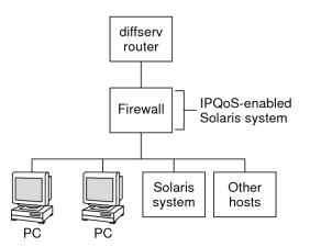
The firewall's security policy determines whether incoming traffic is permitted to enter or depart the internal network. The QoS policy controls the service levels for incoming traffic that has passed the firewall. Depending on the QoS policy, outgoing traffic can also be marked with a forwarding behavior.
