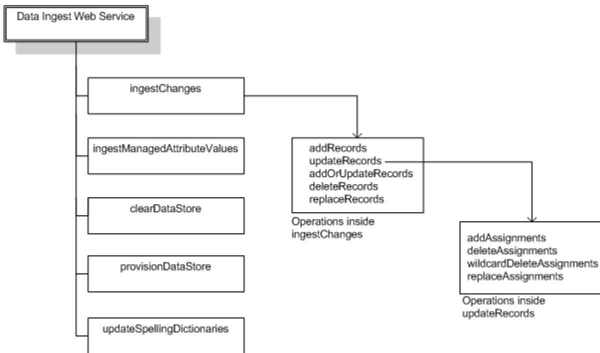
This diagram illustrates the Data Ingest Web Service structure:
