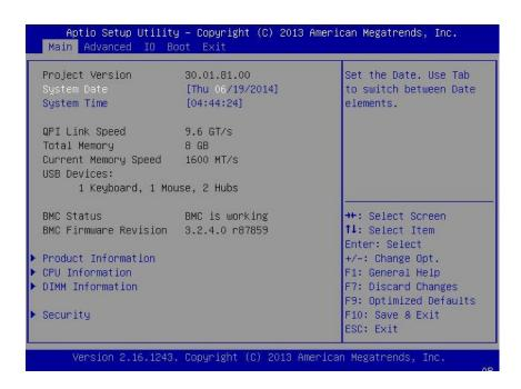
3. Press the F9 key to automatically load the optimal default settings.
