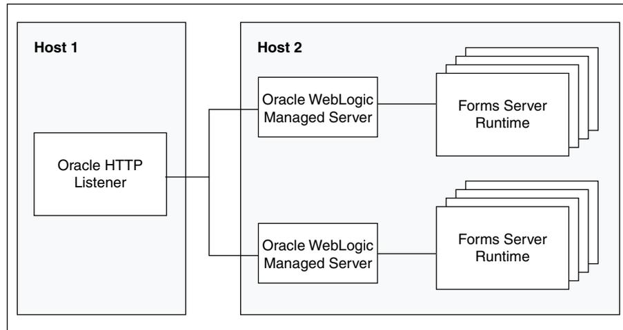
**Figure 5-4 Multiple Oracle WebLogic Servers and multiple Oracle HTTP Listeners on different hosts**
