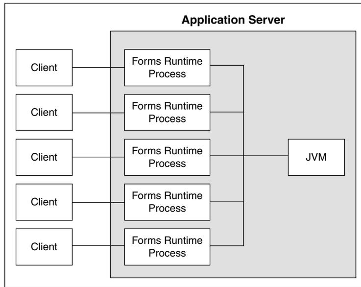
In this example, five clients working in the same application through their own runtime processes are using a pooled JVM process instead of each Forms Runtime process spawning its own JVM instance. This can be a significant savings in memory usage and system resources.
