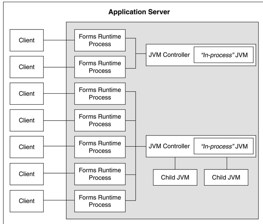
Although it's not shown in [Figure 10-1](#), each JVM controller has a unique name which is used in starting and stopping, or for referencing in the Forms configuration file.
