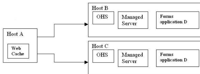
Figure 14–4 assumes a setup where a single Web Cache instance is load balancing two Application Server tiers. This can be described as following:
