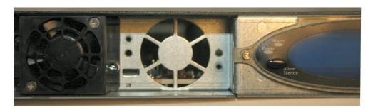
Figure 6-5 Inserting the Fan into the Chassis Slot
