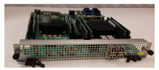
Figure 2-5 Alternate Option Card - Four Port NIU
