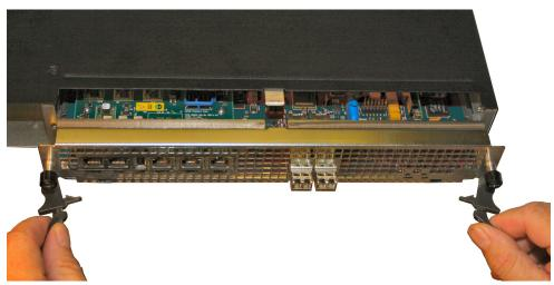
Installing the NIU/TCU (NIU Shown)
