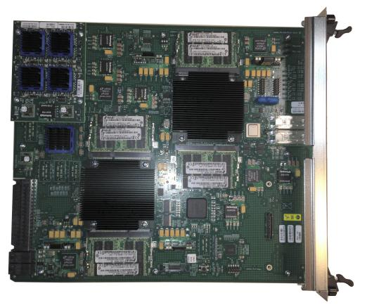
Location of the SSM3 Module (Mounted on Acme Packet 6300/6350)
