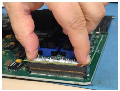
Fully Seating the SSM3 Module Connector
