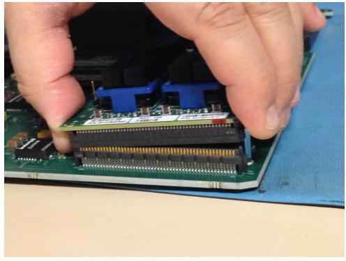
Removing the SSM3 Module
