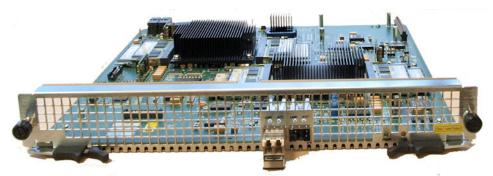
Installed SFP+ Transceiver
