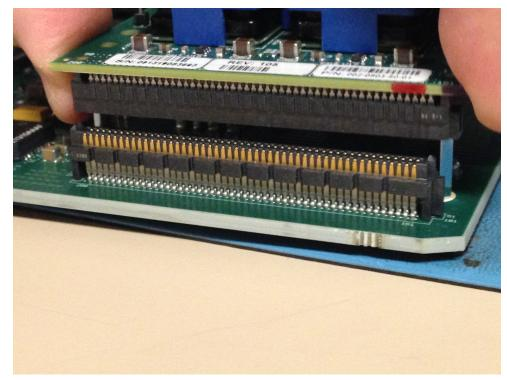
Installing the SSM3 Module
