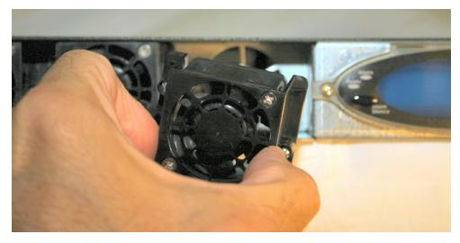
2. Using a small bladed screwdriver, tighten the two captive screws to hold the fan into place.
