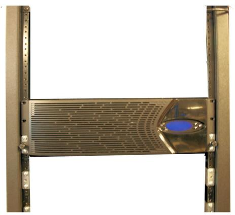
Loosen two thumbscrews securing the Acme Packet 6300/6350 to the Rack
