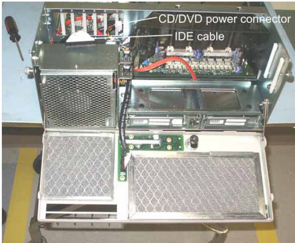
Figure 78: Removable Media Disk Drive Cables (drives removed)
