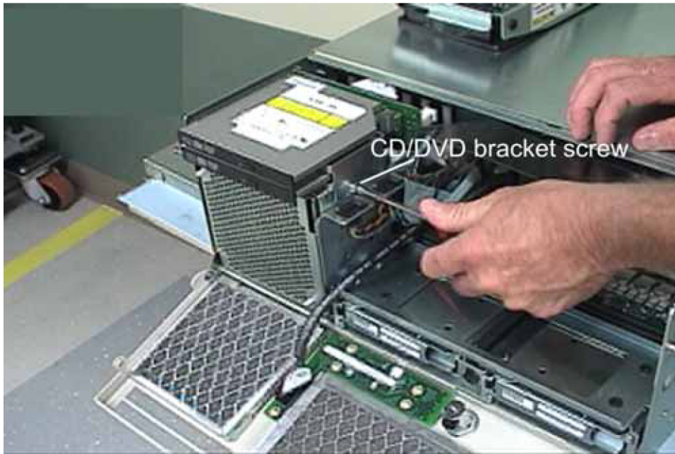
Figure 76: CD/DVD inside bracket screw location
