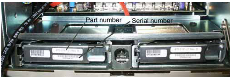
Figure 11: Hard disk label locations
