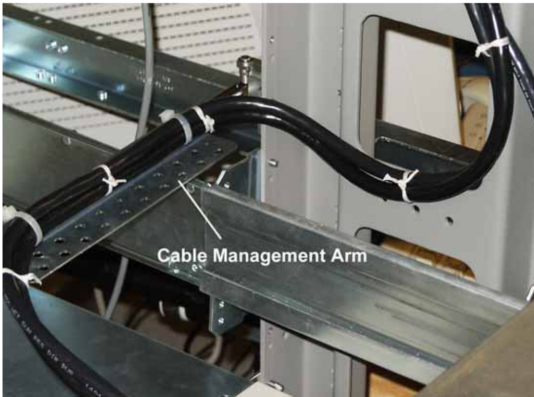
Figure 53: Side Cable Management Arm Installation (T1000 AS shown)
