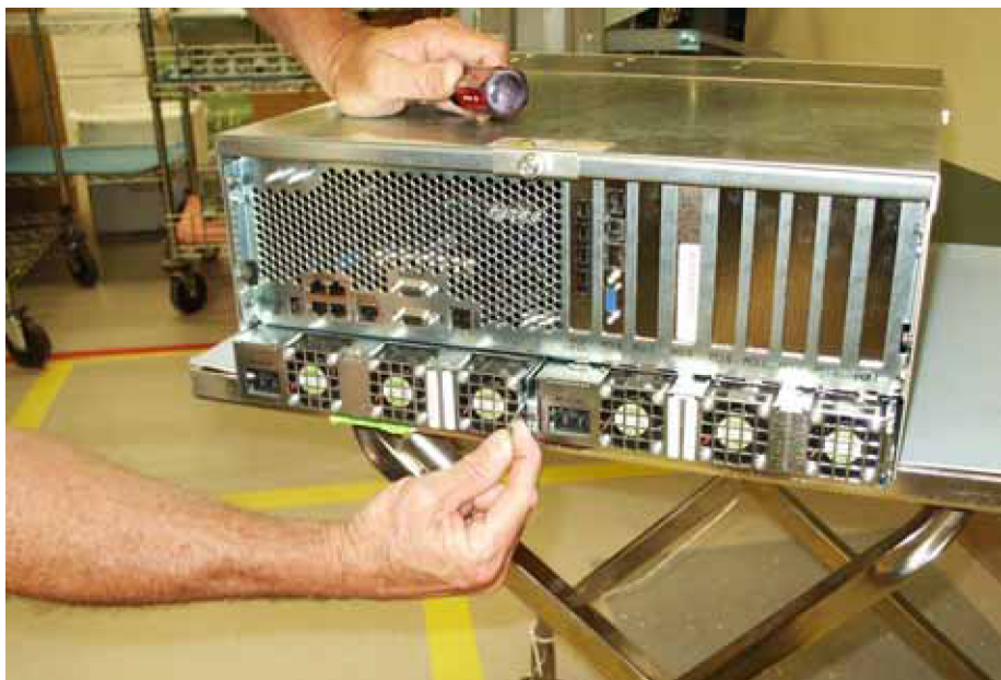
Figure 79: Rotate lock ring down to disengage power supply module.
