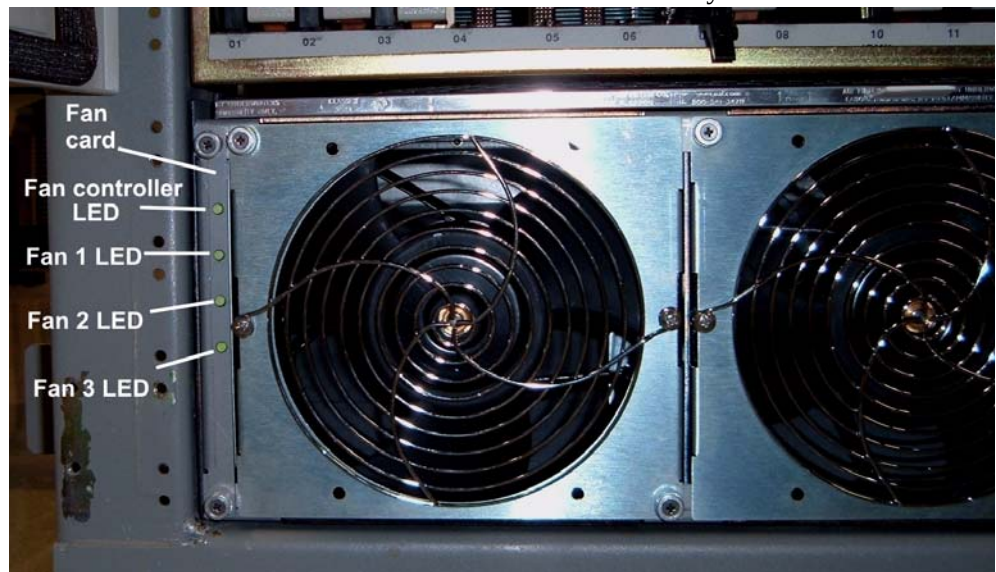
Figure A-24. Fan card with LEDs on front of fan assembly unit
