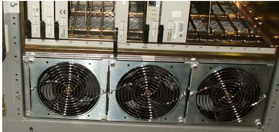
Figure A-26. Fan tray inserted into fan tray bracket in the frame - front view
