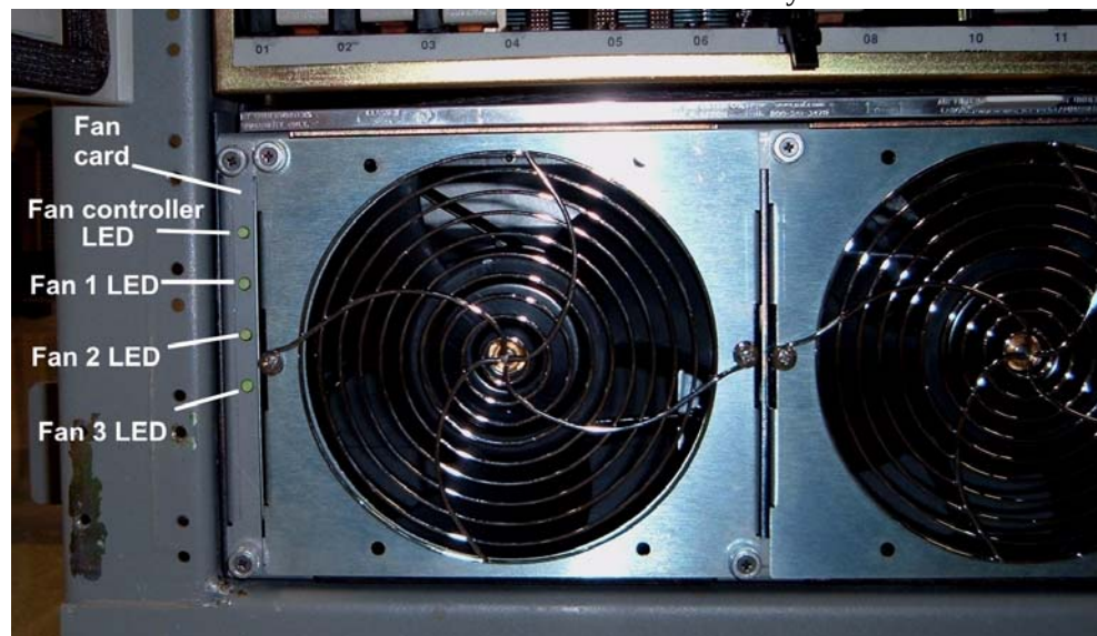
Figure A-29. Fan card with LEDs on front of fan assembly
