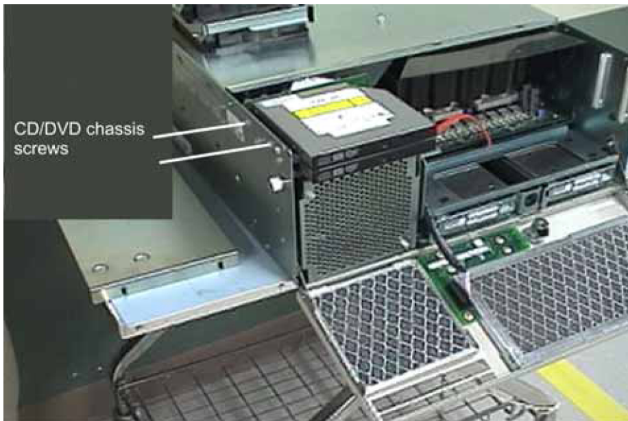
Figure 77: CD/DVD chassis screws
