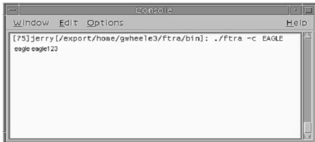
Figure 69. FTRA UNIX Command Line Interface to modify STP data.
