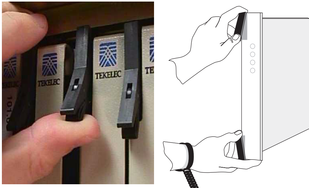
Figure 3-24. Cam-Out/Lock-In Levers on Cards
