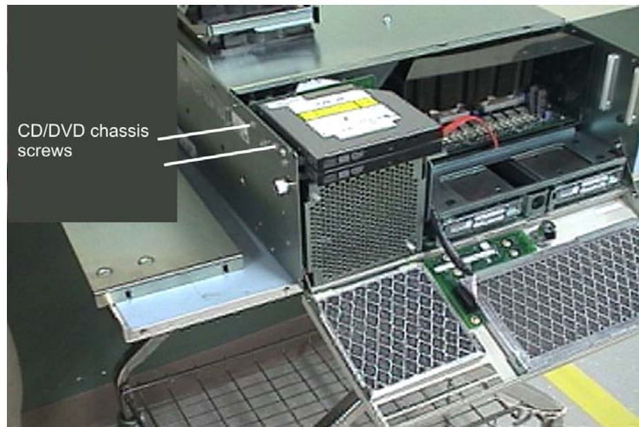
Figure 7-17. CD/DVD chassis screws
