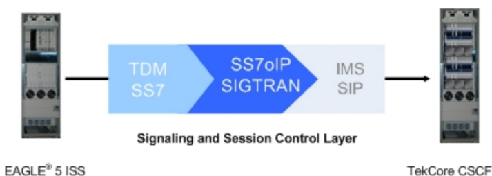
Figure 1-1. Transition from SS7 to IMS
