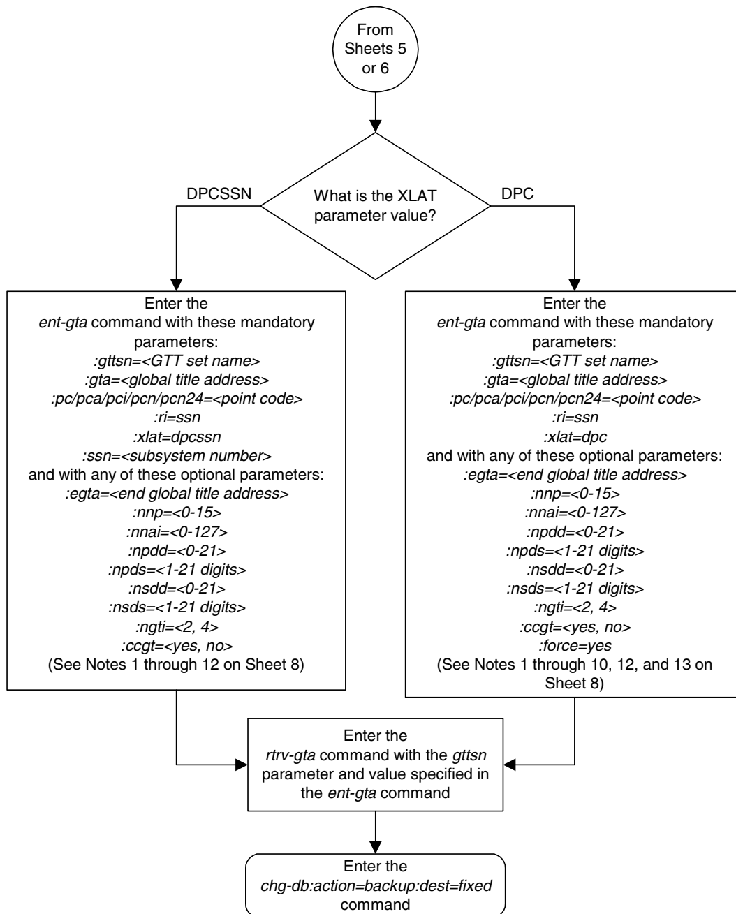
Flowchart 4-6. Adding Global Title Address Information to the Database (Sheet 7 of 8)
