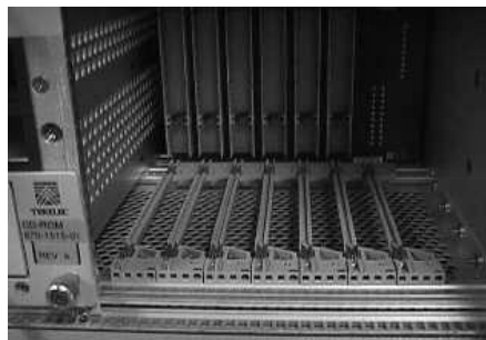
Figure 5-62. EOAP Backplane Connector Pins
