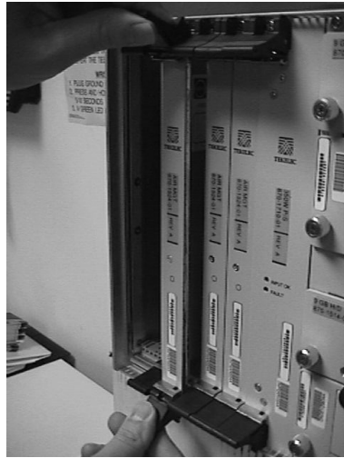
Figure 5-8. Inserting the Replacement Air Management Card
