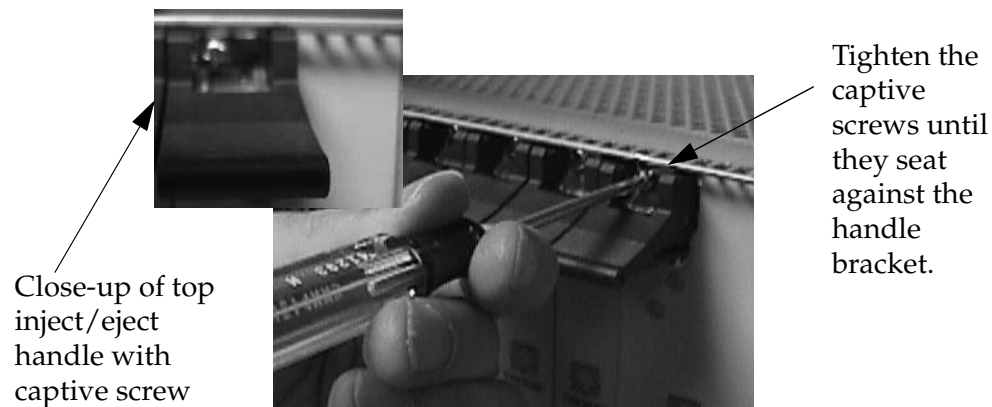
Figure 5-58. Tighten Captive Screws
