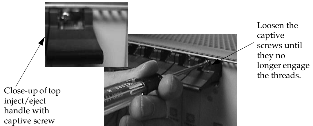
Figure 5-51. Loosening Captive Screws of Power Supply Card
