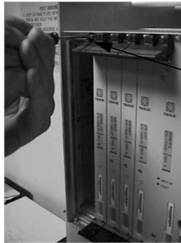
Figure 5-70. Top Handle and Captive Screw of Serial Card
