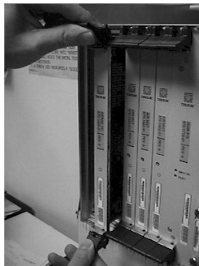
Figure 5-75. Inserting the Replacement Serial Card
