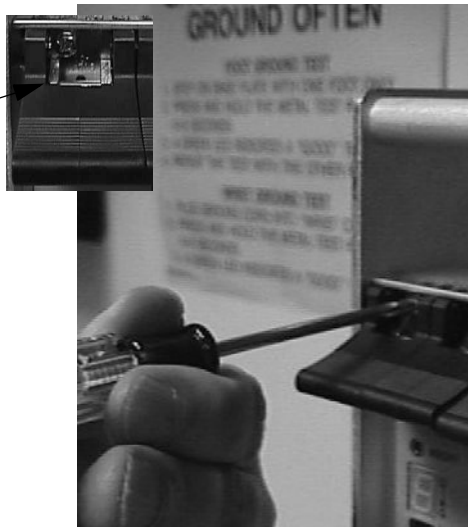
Figure 5-60. Processor Card Captive Screws
