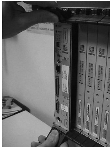
Figure 5-65. Inserting the Replacement Processor Card
