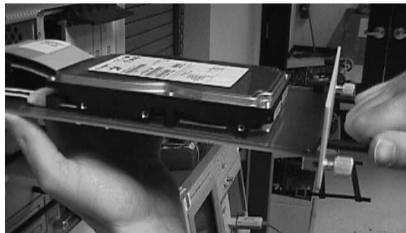
Figure 5-45. Support the Hard Drive Card With Both Hands
