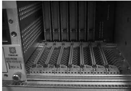
Figure 5-53. EOAP Backplane Connector Pins
