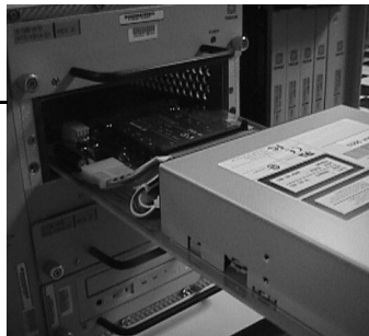
Figure 5-32. Install the CD-ROM Drive Card
