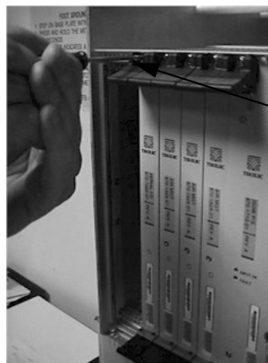
Figure 5-77. Tighten Captive Screws
