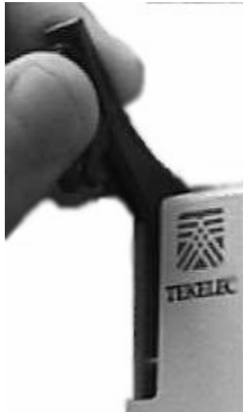
Figure 3-6. Push Inject/Eject Clamps Outward
