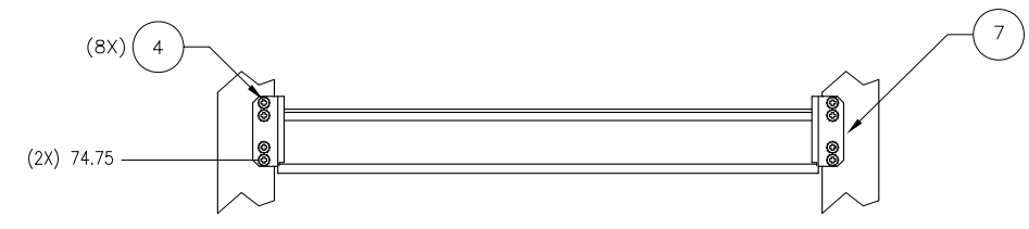
AIR DEFLECTOR POSITION, FRONT VIEW DETAIL C
