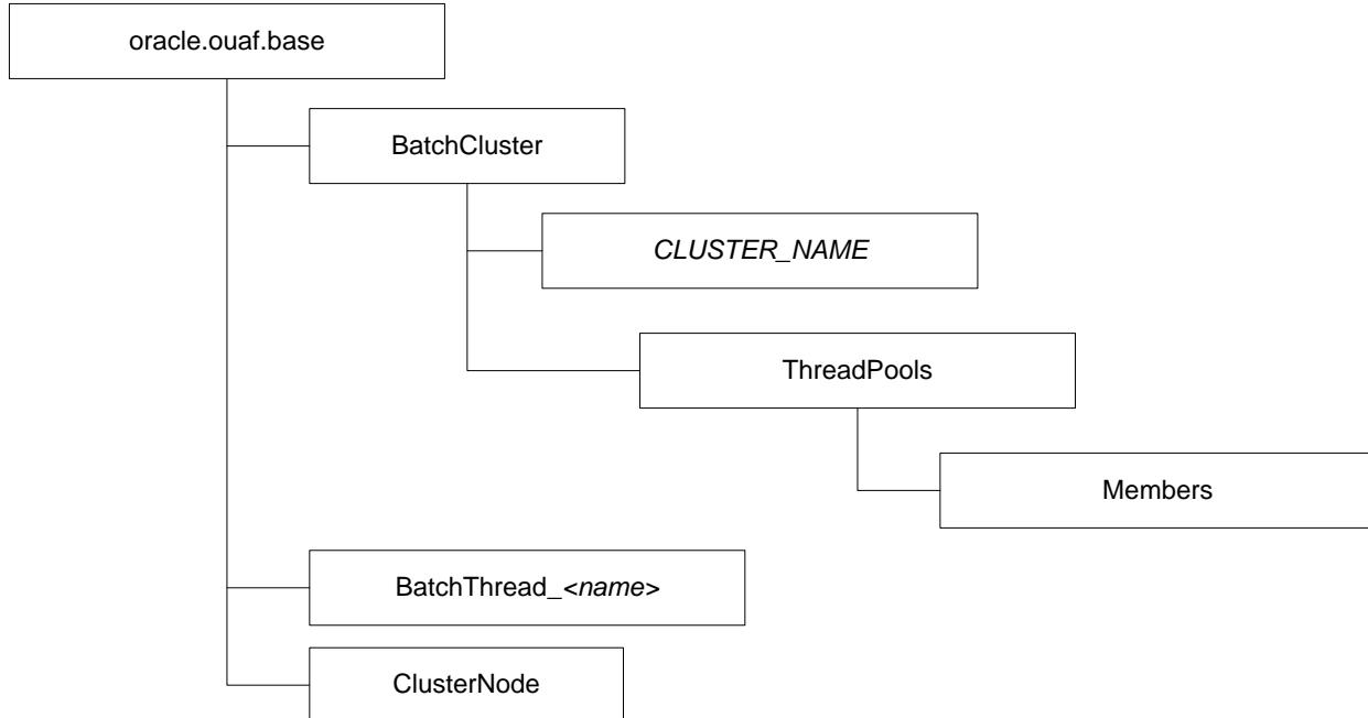
The [BatchCluster MBean](#) holds attributes and operations at the cluster level. The MBean has a series of [Threadpools](#). Each Threadpool has one or more [Members](#) which represent the nodes the threadpool is executing across. Nodes can be present for the same machine or multiple machines (one node per instance).
