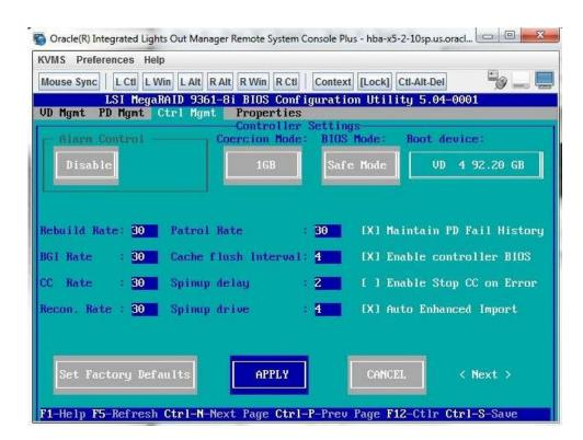
d. Use the arrow keys to navigate to the Apply button, and then press Enter.
