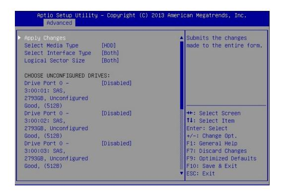
10. In the Drive Selection screen, select the media type, the interface type, and the drives to be included in the RAID configuration.
