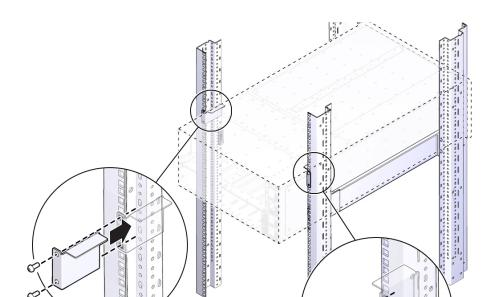
Do not tighten the screws all the way.
