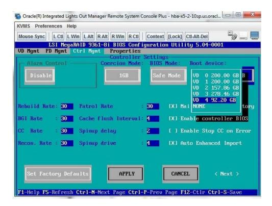
c. Use the arrow keys to navigate to the logical drive you wish to make bootable, and then press Enter.
