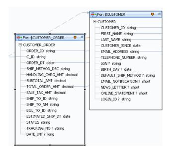
Figure 9–34 Joining tables in the Query Map
