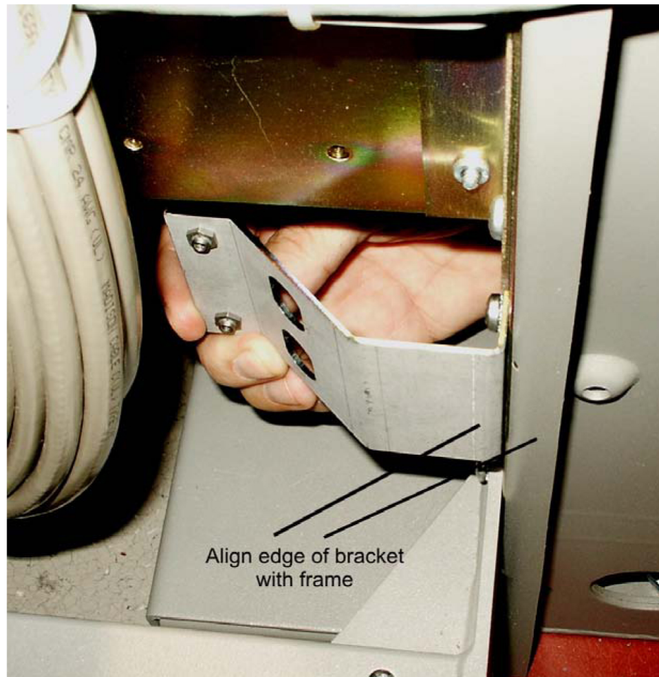
Figure 83: Slide the side fan brackets flush with the Frame
