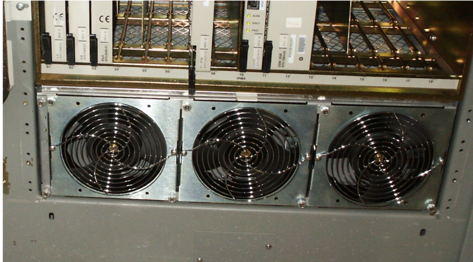
Figure 46: Fan tray inserted into fan tray bracket in the frame - front view
