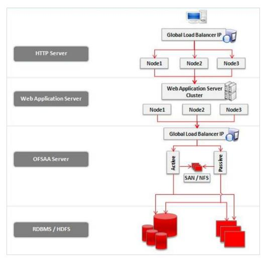
In this diagram, the HA setup is proposed to be ACTIVE-ACTIVE configuration at the HTTP Server, Web Application Server, and Database/ HDFS layers. The OFSAA layer is configured for ACTIVE-PASSIVE configuration.
