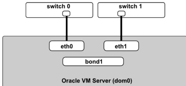
**Figure 5.5 Network bonding for mode 4 with no switch support for VSS or vPC**
