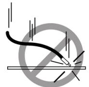
Do not drop the cable or connectors from any height. Gently set the cable down, resting the cable connectors on a stable surface.
