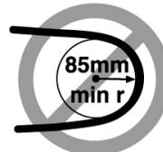
Do not bend the cables to a radius tighter than 85 mm (3.4 inches). Ensure that cable turns are as wide as possible.
