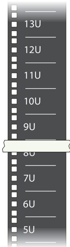
Counting the number of rack units from the bottom of the rack to the mounting location assists you when marking the other rack posts.
