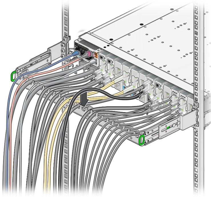
3. **Route the data cables so that they do not interfere with other cables, or with servicing the switch or other systems.**
