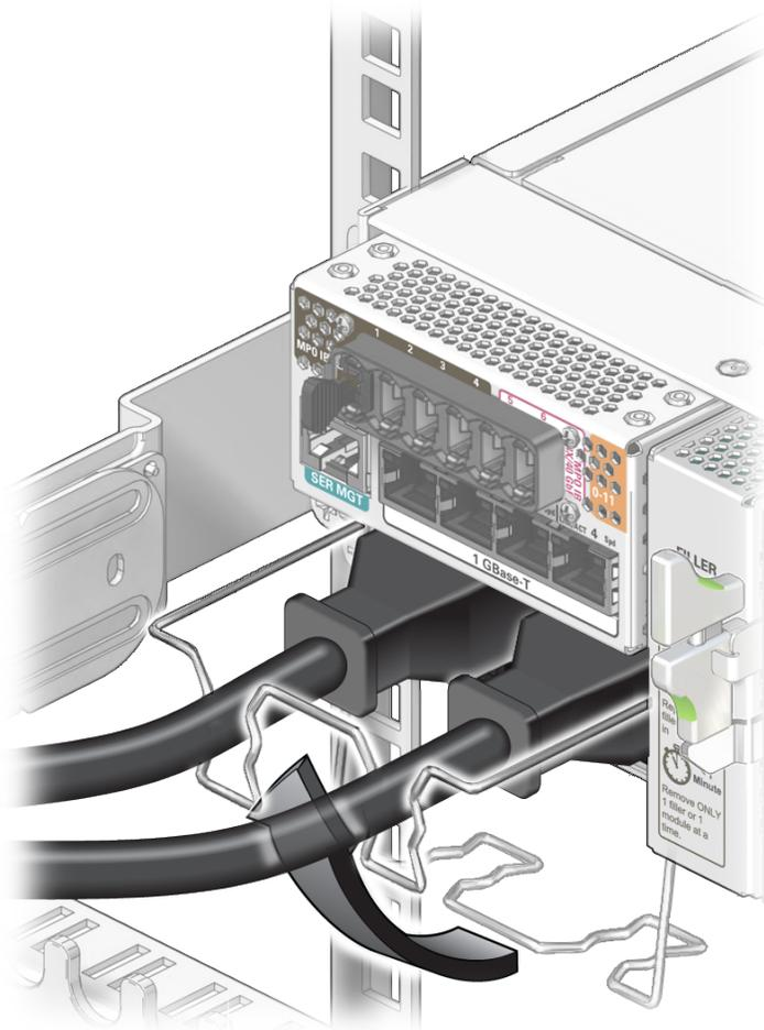
6. **Plug each power cord into the facility power receptacle or power distribution device.**
