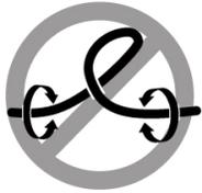
Do not twist the cable to open a kink. If it is not severe, open the kink by unlooping the cable.
