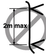
Do not hang the cable for a length more than 2 meters (7 feet). Minimize the hanging weight with intermediate retention points.
