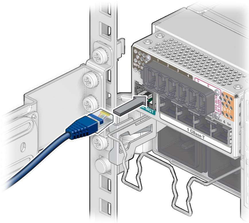
3. **Insert the connector into the receptacle until it clicks, securing it in place.**
