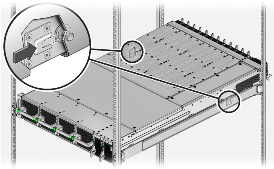
5. **If the screws are not seated in each bracket's slot, slide the switch out far enough to realign the brackets and screws, then slide the switch in again.**
