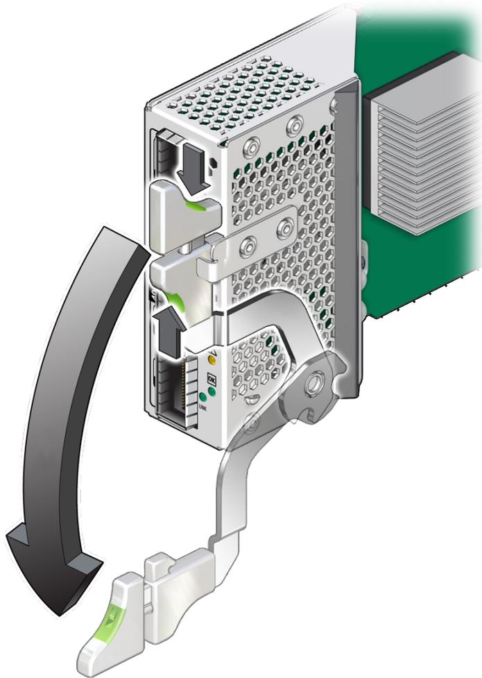
7. **Align the I/O module to the slot where you are installing it.**
