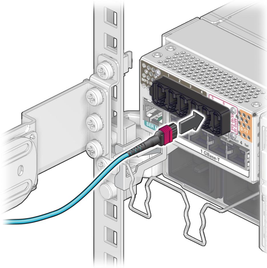
7. Firmly press the PrizmMT connector into the receptacle until you feel the connector securely latch into the receptacle.
