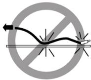
Do not drag the cable or its connectors over any surface. Carry the entire cable to and from the points of connection.
