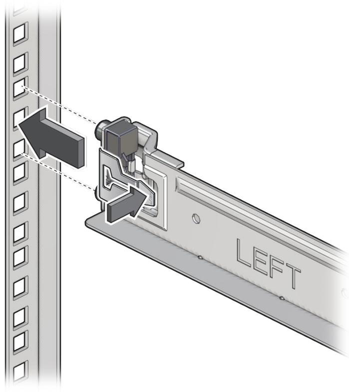
7. **Press the shelf rail into the front rack post while pressing and releasing the release tab.**
