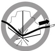
Do not pull the cable out of the shipping box, through any opening, or around any corners. Unroll the cable as you lay it down and move it through turns.
