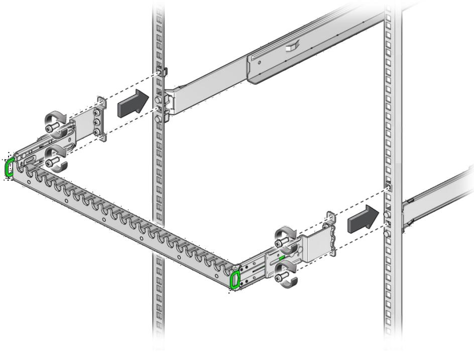
3. Using a No. 2 Philips screwdriver, secure the upper mounting holes of the cable management comb to the 10-32 cage nuts with two 10-32 screws.
