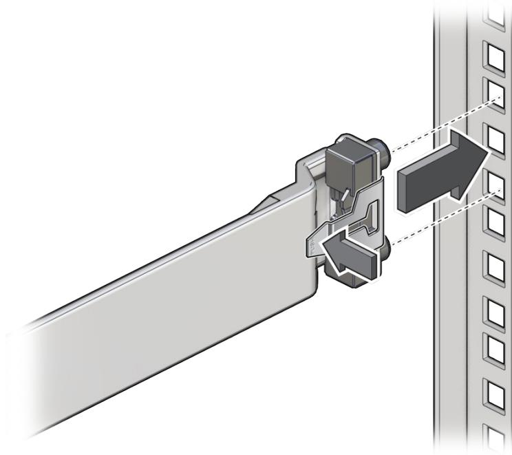
5. **Press the shelf rail into the rear rack post while pressing and releasing the release tab.**
