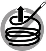
Do not uncoil the cable, as a kink might occur. Hold the coil closed as you unroll the cable, pausing to allow the cable to relax as it is unrolled.
