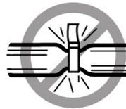
Do not cinch the cable with hard fasteners or cable ties. Use soft hook-and-loop fastener for bundling and securing cables.
