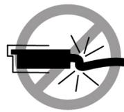
Do not force the cable connector into the receptacle by pushing on the cable. Apply connection or disconnection forces at the connector only.
