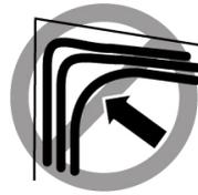
Do not pack the cable to fit a tight space. Use an alternative cable route.
