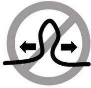
Do not straighten the cable to correct a bend that is too tight. Leave the cable bend as is.
