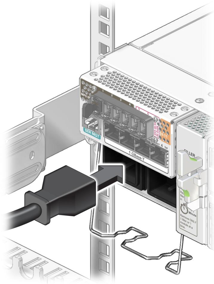
5. **Raise the retaining wire back up and snap it over the power cords to secure them.**
