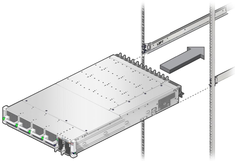
4. **While sliding the switch into the rack, on each side of the switch, make sure each mushroom screw slips into the slot in its bracket.**
