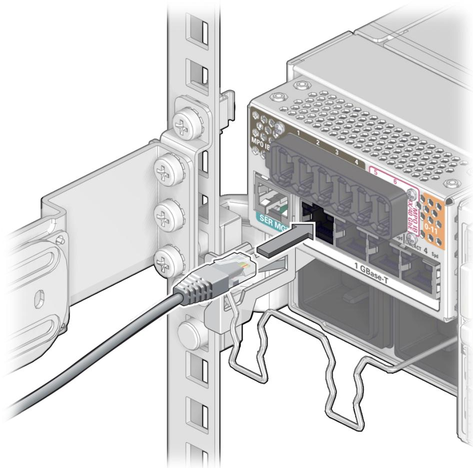
For the Oracle F2 Quad Port 10GBASE-T module, the tab on the connector is to the right.
