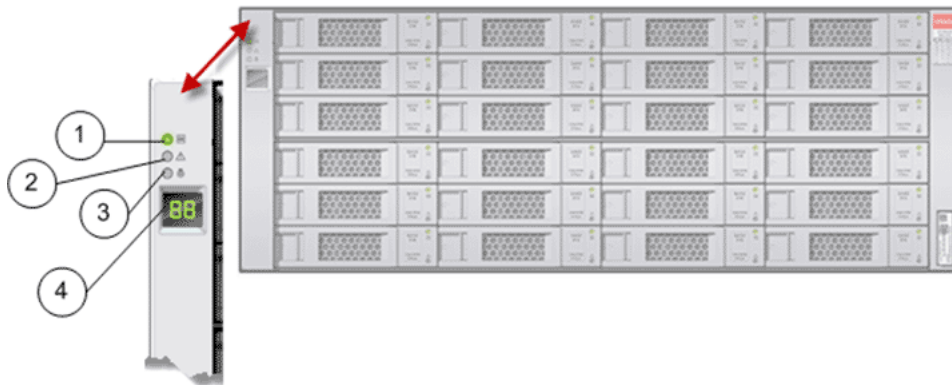
Figure 198: Operator panel LEDs (DE2-24C Drive Enclosure)
