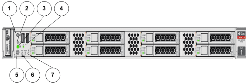
Figure 203: LEDs at the front of the Pilot
