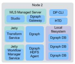
In a two-node configuration, all Hadoop components and the Data Processing libraries are hosted on one node, while the remaining BDD components are hosted on the other. Although the diagram above shows the Dgraph databases stored on the local file system, they could also be stored in HDFS on Node 1.
