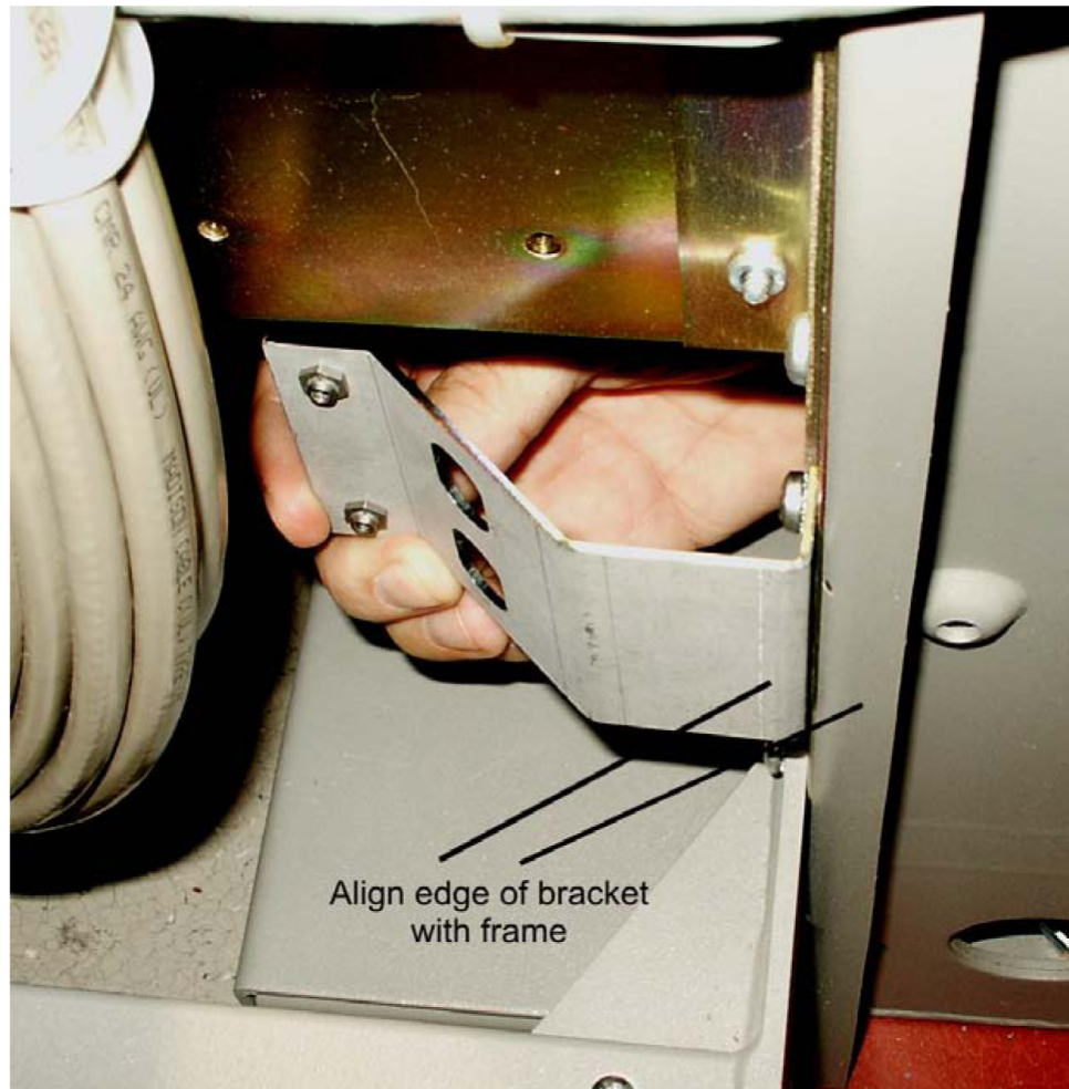
Figure 6-15 Slide the side fan brackets flush with the Frame
