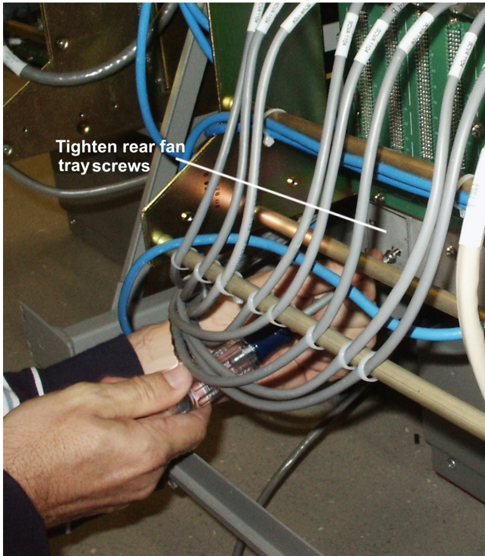
Figure 6-21 Tighten rear fan tray screws
