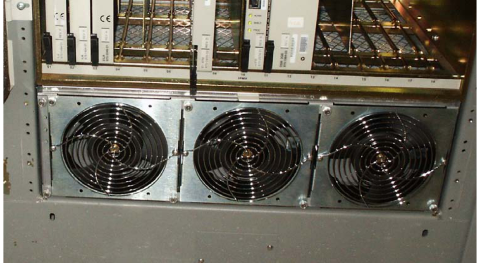
Figure 6-20 Fan tray inserted into fan tray bracket in the frame- front view
